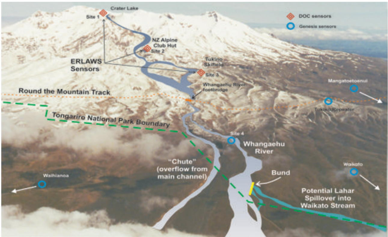
Above: Graphic showing the location of the ERLAWS sensors (DOC and Genesis), the bund and the likely path of the lahar from Crater Lake.
