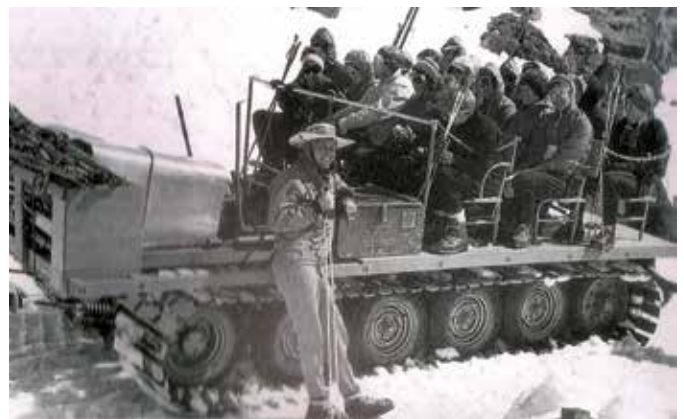
The 'Whakapapa Cat', designed and built by Tom and Jim Bates in the early 1960s to carry skiers and sightseers from the topmost lift at Whakapapa to the Col above Crater Lake. Photo: Arthur Bates
