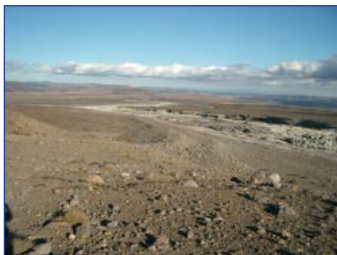
Figure 4. Helicopter view during the lahar event on 18 March 2007 looking downstream with the bund on the left. The photo was taken during rain just after peak flow and shows how the edge of the flow ran along the foot of the sacrificial apron for about half its length.
