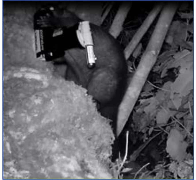
Figure 5: Possum attempting to unscrew Chirp head off Goodnature A24. Photo: Nick Green
