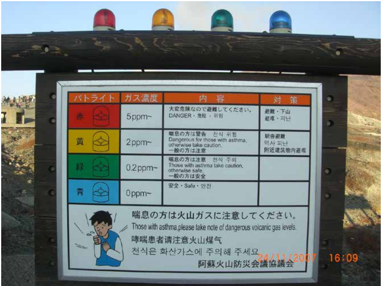
Figure 3: Gas warning system for the public on the rim of Nakadake crater, Asosan volcano. Photo: Harry Keys
